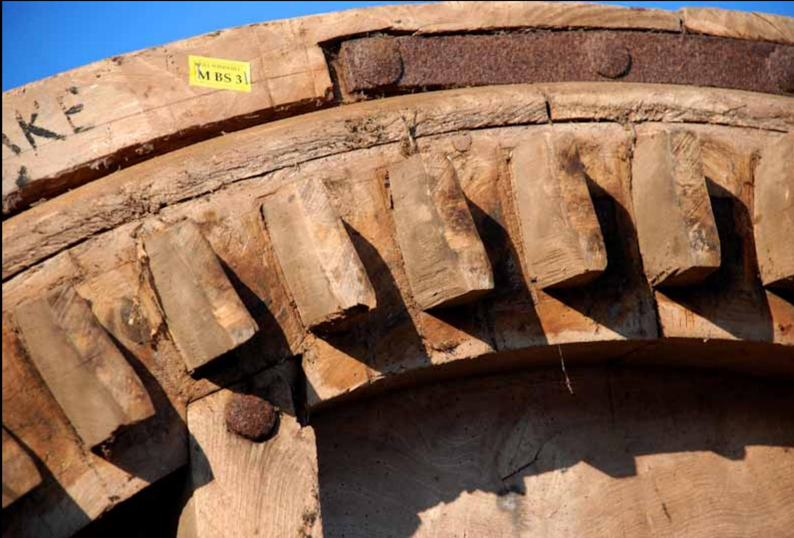
The yellow tag that can be seen is just one of over 500 unique identification labels that have been used to record every mill piece and its position and location within the mill
